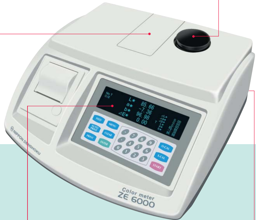
Measurement by setting color samples on a measuring stage
