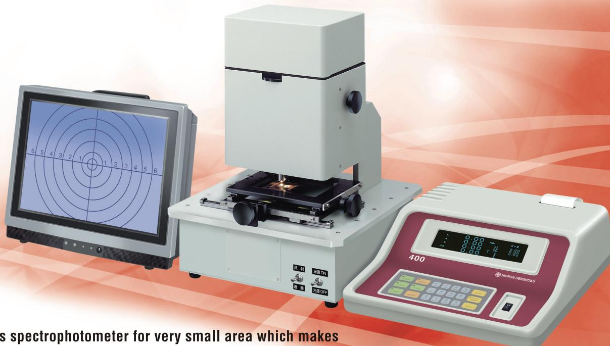
This model is spectrophotometer for very small area which makes it possible to measure the spectral reflection rate and spectral transmittance by magnifying the microscopic area through a microscope. The measuring area is projected on the monitor and you can check the area and focus on the measuring area till 0.05mm.
